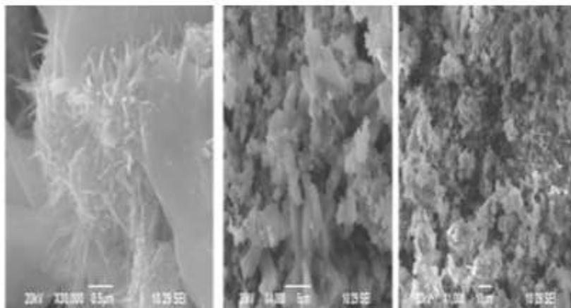
**Figure 4.** SEM images of  $\text{Co}_3\text{O}_4$ .
