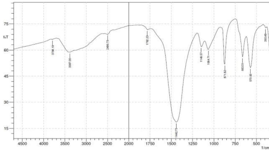
**Figure 2.** IR spectrum of  $\text{Co}_3\text{O}_4$  nanoparticles.
