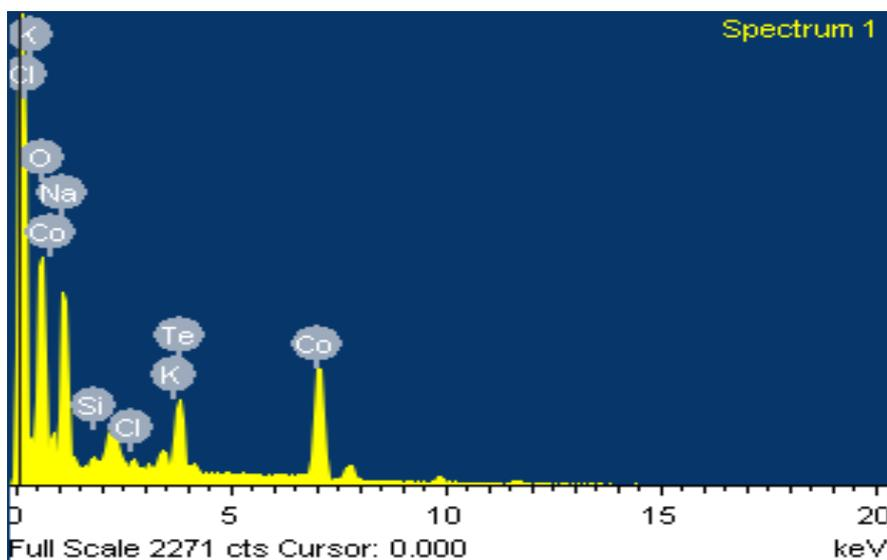
**Figure 5.** EDX of spectra of  $\text{Co}_3\text{O}_4$ .
